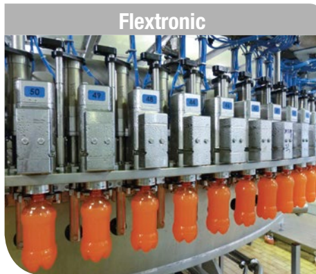
Flextronic Extremely innovative and flexible platform of electronic volumetric fillers suitable to handle to still or carbonated, clear or pulpy and hot or cold-fill products, and weight filling.
