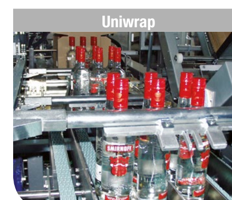
Uniwrap Wrap-around cartoning machines with continuous movement. Patented system for partition insertion available upon request.
