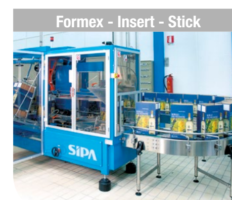
Formex - Insert - Stick Complete cartoning lines for carton erection and closure, also with partitions.
