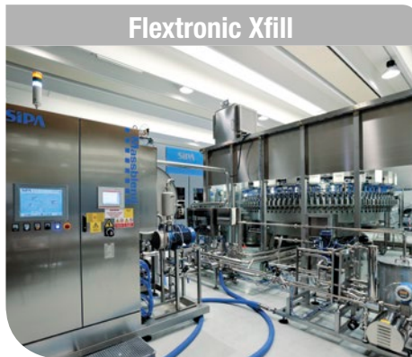
Flextronic Xfill Innovative configuration with the integration mixer-filler: No on-board product tank for carbonated products filling, the mixing unit buffer tank is used as a product tank for the filler.
