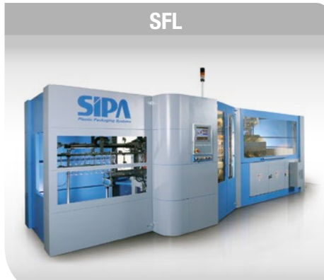
SFL Linear Blowmolders. Output from 500 to 10,800 bottles/hour.
