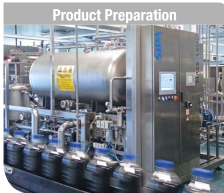
Product Preparation Degassing and carbonation unit, blending and carbonation unit with massic control, C.I.P. unit, continuous in-line multi-components blending unit, product pasteurization unit, product carbonation unit.
